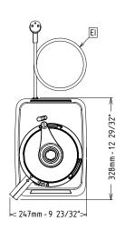
Electric Supply voltage: 220-240 V/1N ph/50/60 Hz Electrical power max.: 0.75 kW 0.75 kW **Total Watts:** Capacity: Performance (up to): Capacity: 2.6 litres Key Information: External dimensions, Width: 247 mm External dimensions, Depth: 328 mm External dimensions, 456 mm Height: **Shipping weight:** 18.7 kg Meat mincing capacity: 0 kg Mayonnaise preparation 0 kg capacity: **Pastry preparation** capacity: 0 kg
